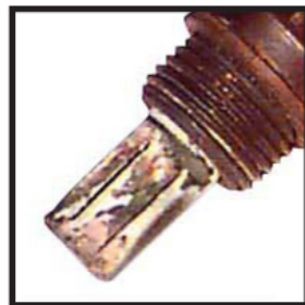
Ethylene Glycol (Antifreeze) Contamination
