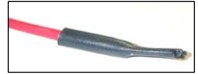
Correct unused lead termination
